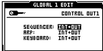
The parameter in this window control where data should be sent from the internal Sequencer, the Arpeggiator and the **Keyboard** (only functional on the SFX-6). Joystick control is included in the Keyboard parameter. The available selections are:
