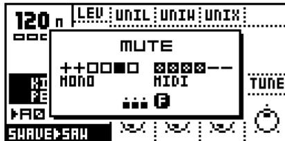
If you press the [TRIG] keys while holding [FUNCTION] the mute change is held until [FUNCTION] is released. A track that is currently muted but will be un-muted when [FUNCTION] is released is displayed as a “+” sign. A track that is currently not muted but will be muted when [FUNCTION] is released is displayed as an “X” sign.
