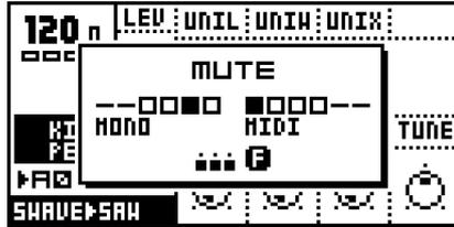
In addition to the <TRIG> LED's, the Mute-state is also indicated in the Mute window. Boxes means that the track is un-muted, and a dash means it is muted. The <TRACK> LED's will also be updated.
