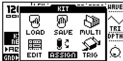
You find the Assign window in the Kit menu. Press the **[KIT]** key and navigate to the Assign icon using the **[CURSOR]** keys, then press **[ENTER/YES]** to enter the Kit menu.
