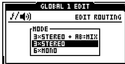
The **3xSTEREO** is the default configuration, where the three internal stereo mix buses AB, CD and EF are sent to the audio outputs A/B, C/D and E/F.
