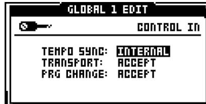
The tempo can be generated either internally or taken from an external MIDI clock. The Monomachine gives best timing performance when set to internal synchronisation. It transmits a very high precision MIDI clock on the MIDI OUT port so that you can synchronise other devices to the Monomachine.
